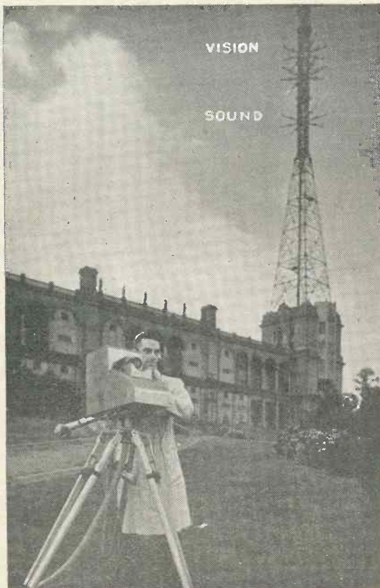
The Marconi-E.M.I. Emitron electron camera being used in the grounds of the Alexandra Palace.
